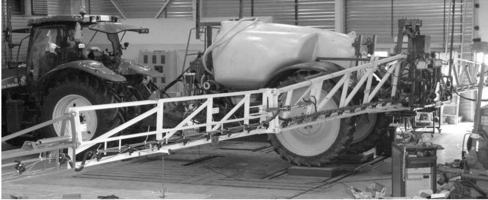
Figure 1: Picture of the tractor-trailer-sprayboom combination on the shaker
