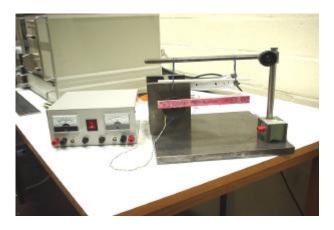
Figure 5: Experimental test set-up with the suspended IPC test beam.
