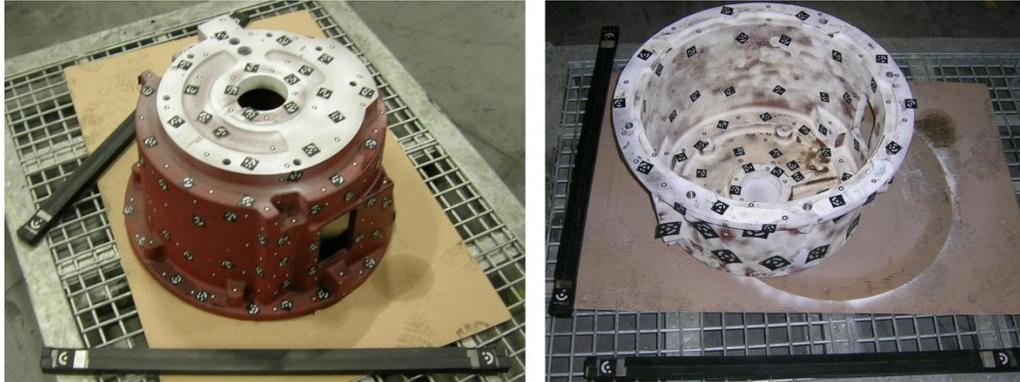
**Fig. 2 Images showing the lantern housing during the digitizing process.**
