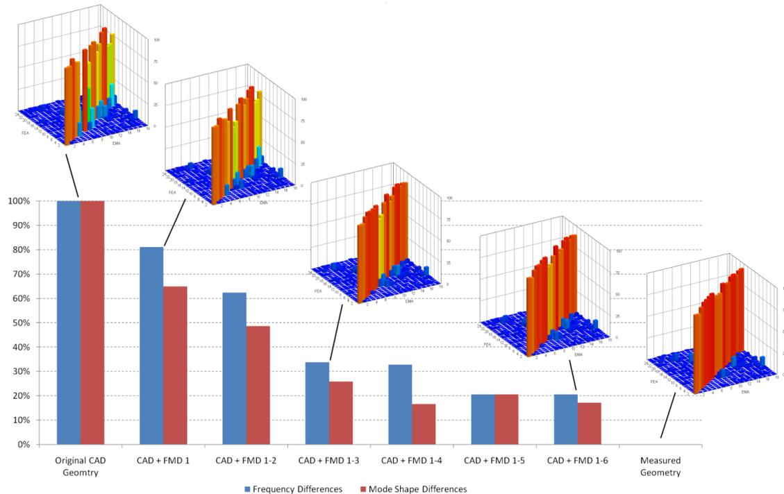
**Fig. 9 The impact of the geometry modifications on the modal correlation**
