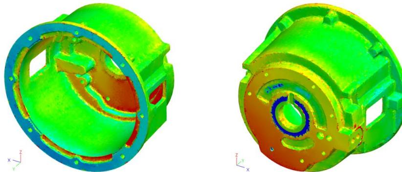
**Fig. 6 The difference between the measured and CAD geometry.**
