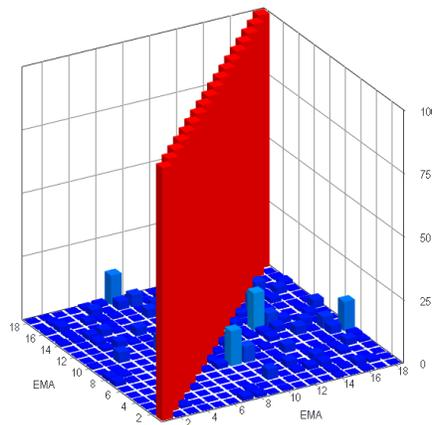
**Fig. 5 The AutoMAC of the measured mode shapes**
