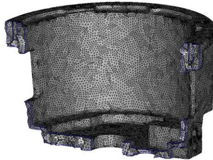
**Fig. 4 Resulting 10-noded tetrahedron mesh**
