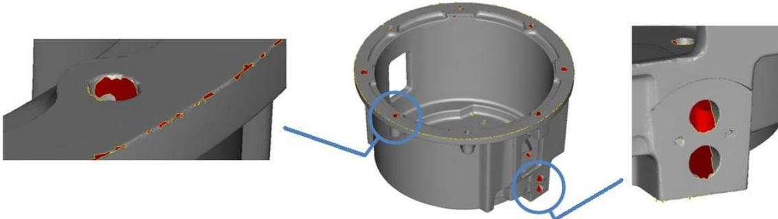
**Fig. 3 Detail views of typical scan surface mesh imperfections: non-watertight edges (left) and incomplete hole or slot information (left and right).**
