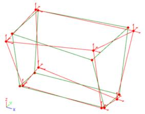
Error estimation using rigid body mode comparison of the equivalent homogeneous brick.
