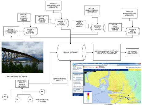
Figure 1: BCSIMS System Architecture:
