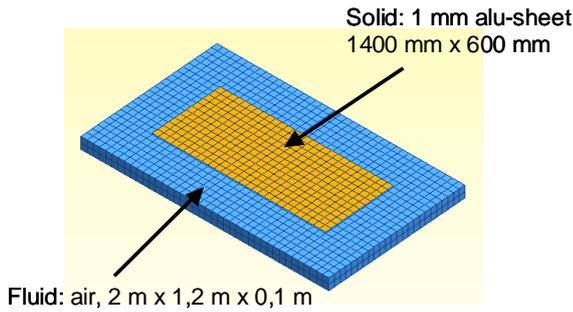
Fig.1 FE-model of a plate resonator coupled to a fluid volume
