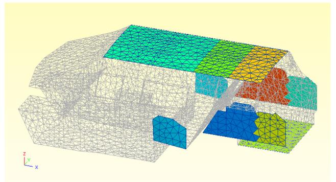
Fig.7 FE-Model of a car interior with plate resonators
