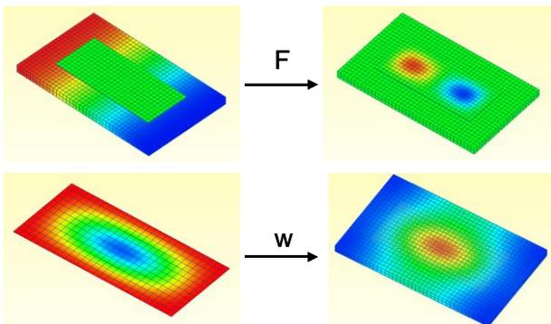
Fig.2 Generation of MAM, top: static deflection shape of the plate resulting from the pressure field of mode 1 of the
