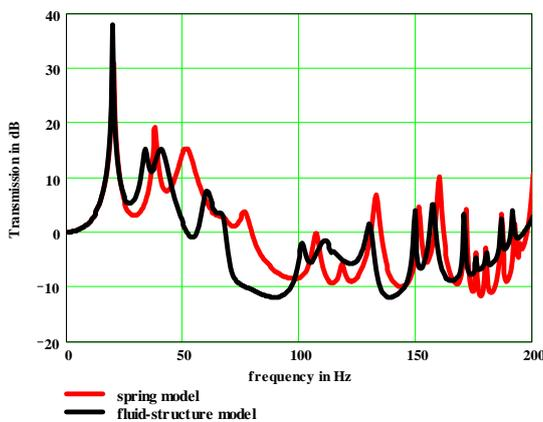
Fig.5 Spectra of transmission of structure borne sound in dB, comparison of an FSI-model and a substitute model with spring elements
