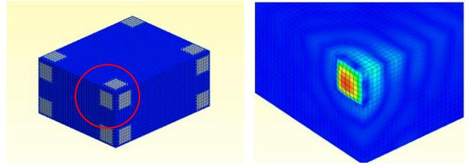
Fig.6 FE-model of a reverberation chamber with 12 possible resonator positions (left) and one orthogonalized "static" MAM of the fluid component.
