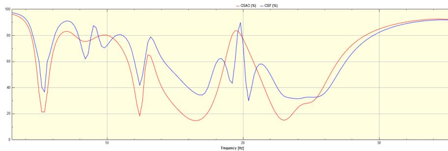
**Figure 8: The CSAC (red) and CSF (blue) FRF correlation functions for the initial parameter values.**
