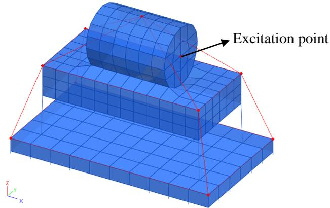
**Figure 2: The measurement grid**
