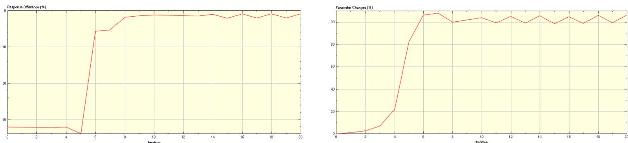
**Figure 9: The iteration history of the CSF response at 8.0 Hz (left) and the  $K_z$  of the connection springs (right).**
