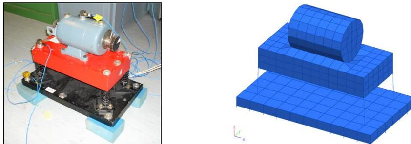
**Figure 1: The considered test set-up (left) and the FE-model (right).**
