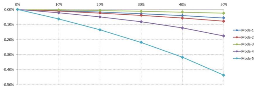
**Fig. 7 Illustration of the non-linear relation between the resonant frequencies and the level of damage.**
