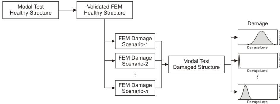
**Fig. 1 The scenario-based damage identification technique.**
